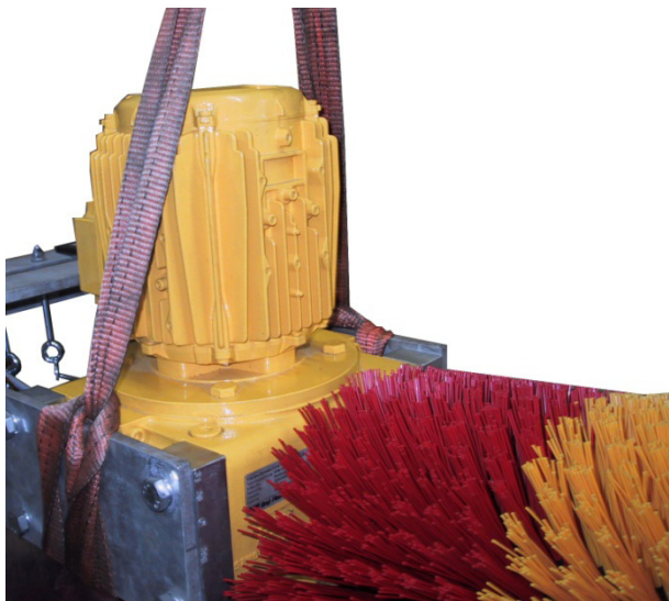
Figure 3: Affixing the lifting harness
